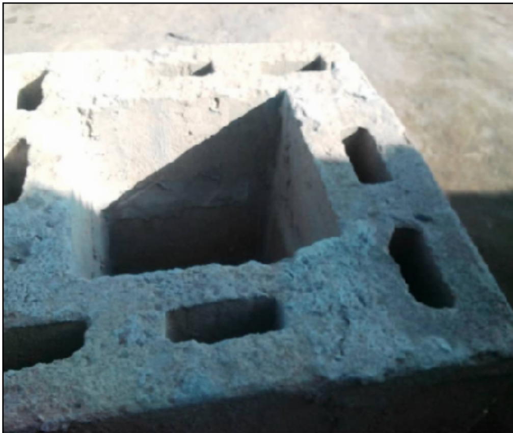
THIS IS A 6 INCH BLOCK FORM WHICH WILL MAKE THE INSIDE COLUMNS
