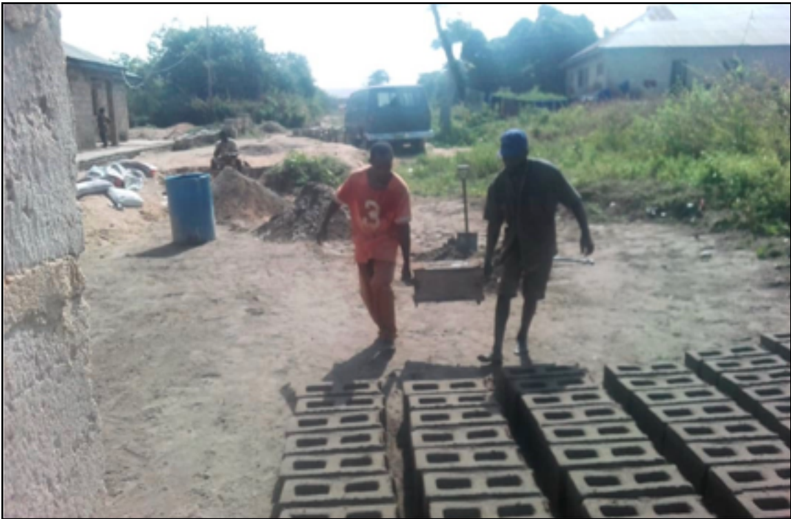
AFTER THE BRICKS ARE FORMED, THEY ARE PLACED IN ROWS TO DRY.
