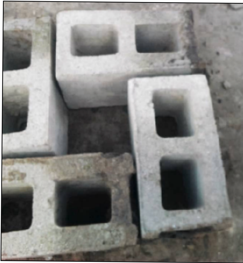
AREMU WAS SHOWING ME THAT THE 9 INCH BLOCKS WOULD BE TOO BIG FOR AN INSIDE COLUMN
